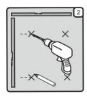
Mark the spots on the wall at which the brackets will be mounted. Drill the holes of required diameter, 40 mm in depth. Place the plastic dowels into the holes. Affix brackets to the wall using bolts.
