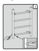
Fix radiator to the brackets. Position the drying bracket at the mounting spot and use the connectors to attach it to the heating system. Fasten the drying brackets with the screws.
